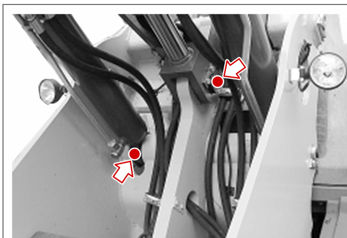
Lubrication point on the lifting cylinders - bottom and a lubrication point on the compensation cylinder (rod-side).
