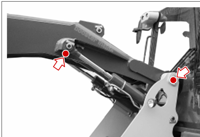
Lubrication points on the frame and lifting cylinder - rod-side (both sides)
